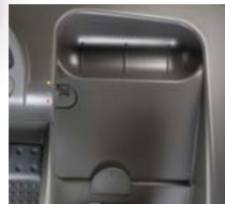
Desk Pad - provides convenient recessed holding areas for clipboards, pens and small tools.
