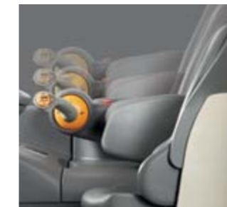
Adjustable Armrest, Control Handle and Seat - enhance comfort and control with individual settings.
