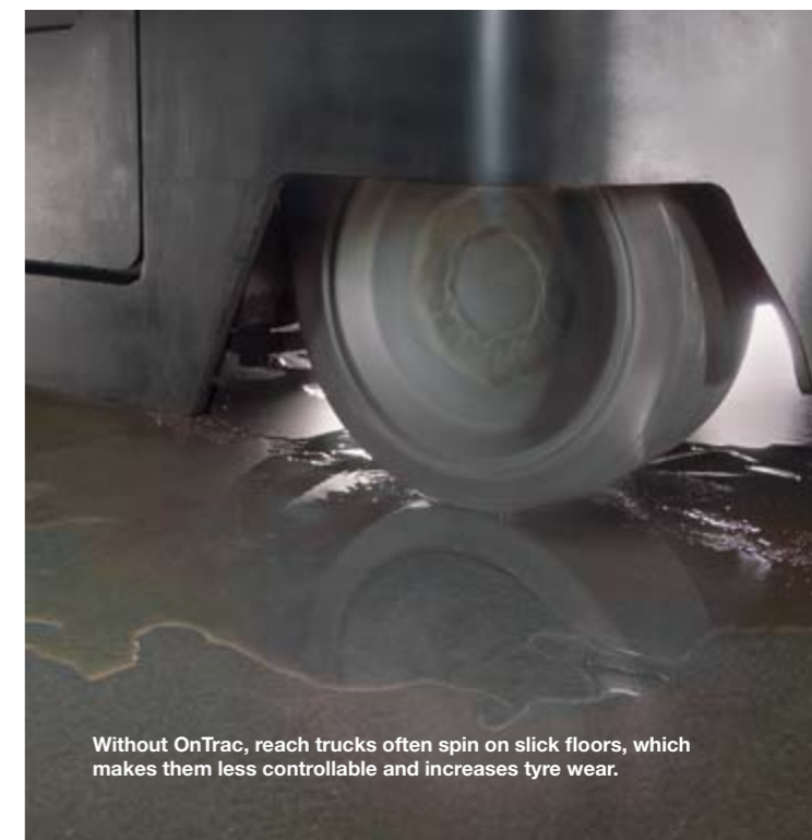
OnTrac™ Anti-Slip Traction Control reduces tyre spin and provides maximum available traction during acceleration, plugging and braking by monitoring changing conditions.
